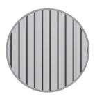
Round tube section infill ø 25mm welded to the structure.
