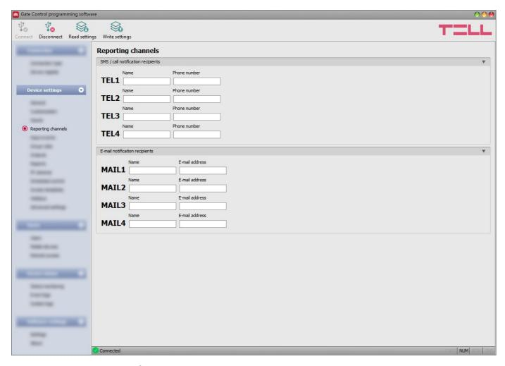
In this menu you can configure the telephone and e-mail availabilities, to which you want to send notifications about events generated by triggering the **IN1...IN4** contact inputs.
