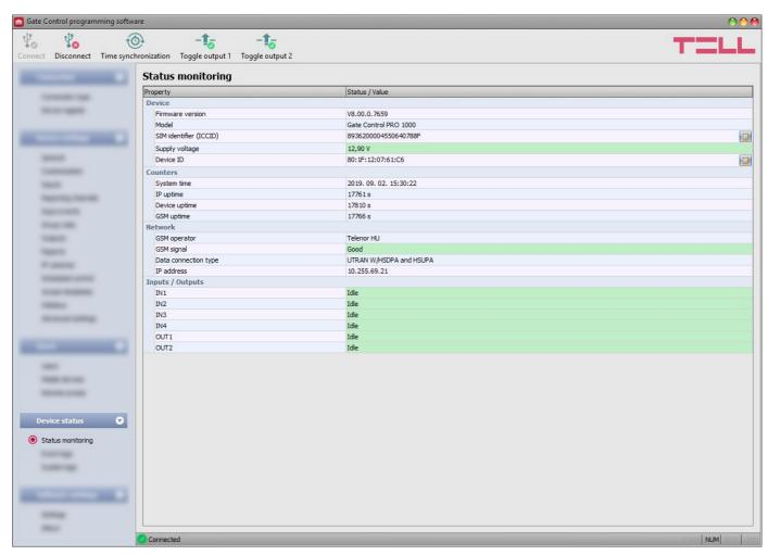
In this menu you can read information about the actual system status. Status information is read from the device and refreshed automatically only when connected through USB. When connected remotely, you can read and refresh the status information by clicking on the "*Read*" button. The availability of certain status information listed below depends on the connected device model.
